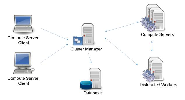
The deployment may consist of five distinct components: the *Clients*, the *Cluster Manager*, the *Database*, the *Compute Server nodes*, and the *Distributed Worker nodes*. Several of these are optional, and a few can be replicated for high
